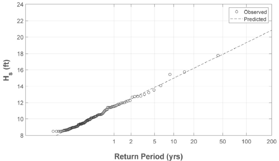
Figure 1-5. Extreme Wave Analysis 1998-2019 (CDIP Station 045) (CFC, 2019)
