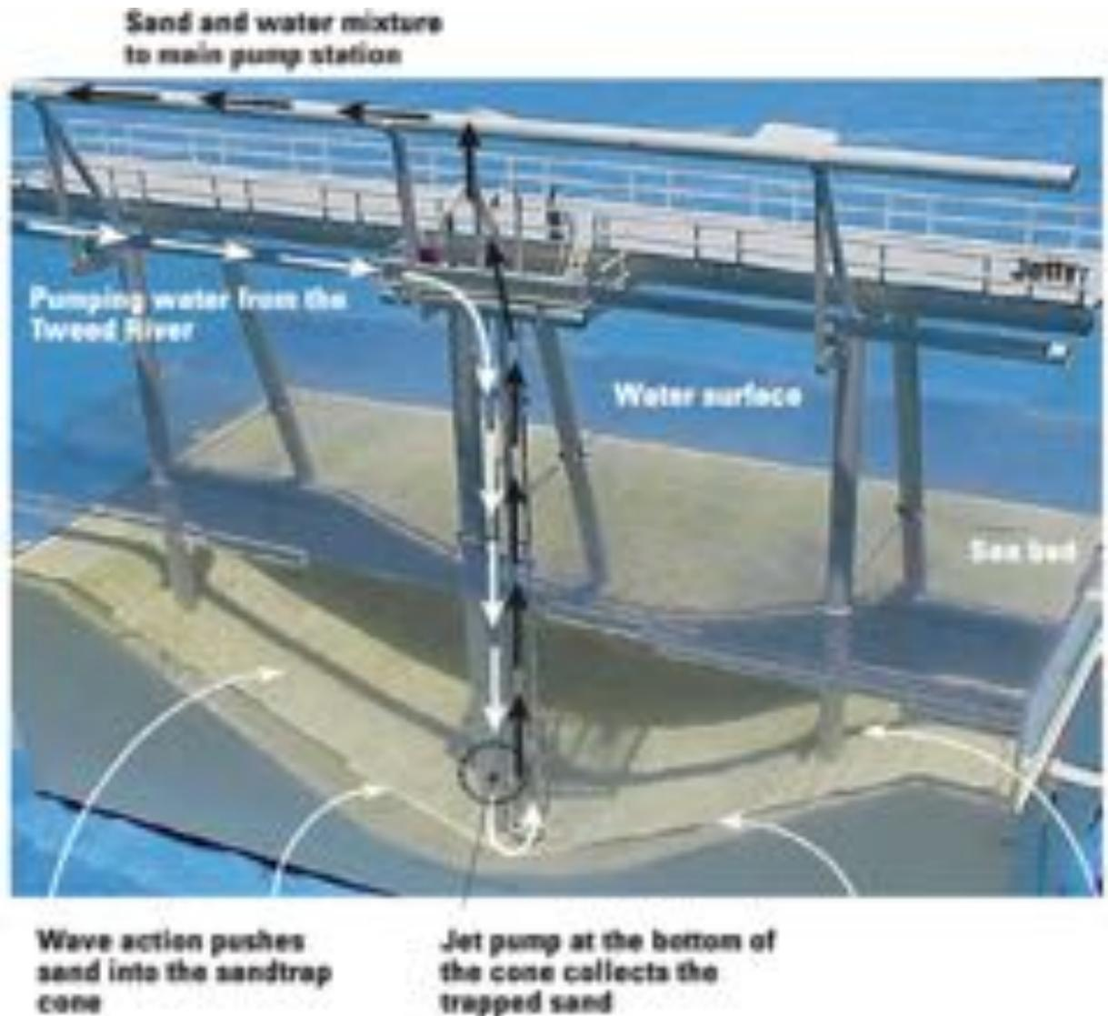
**Figure 2-18. Tweed Sand Bypass Intake System (GHD, 2011)**
