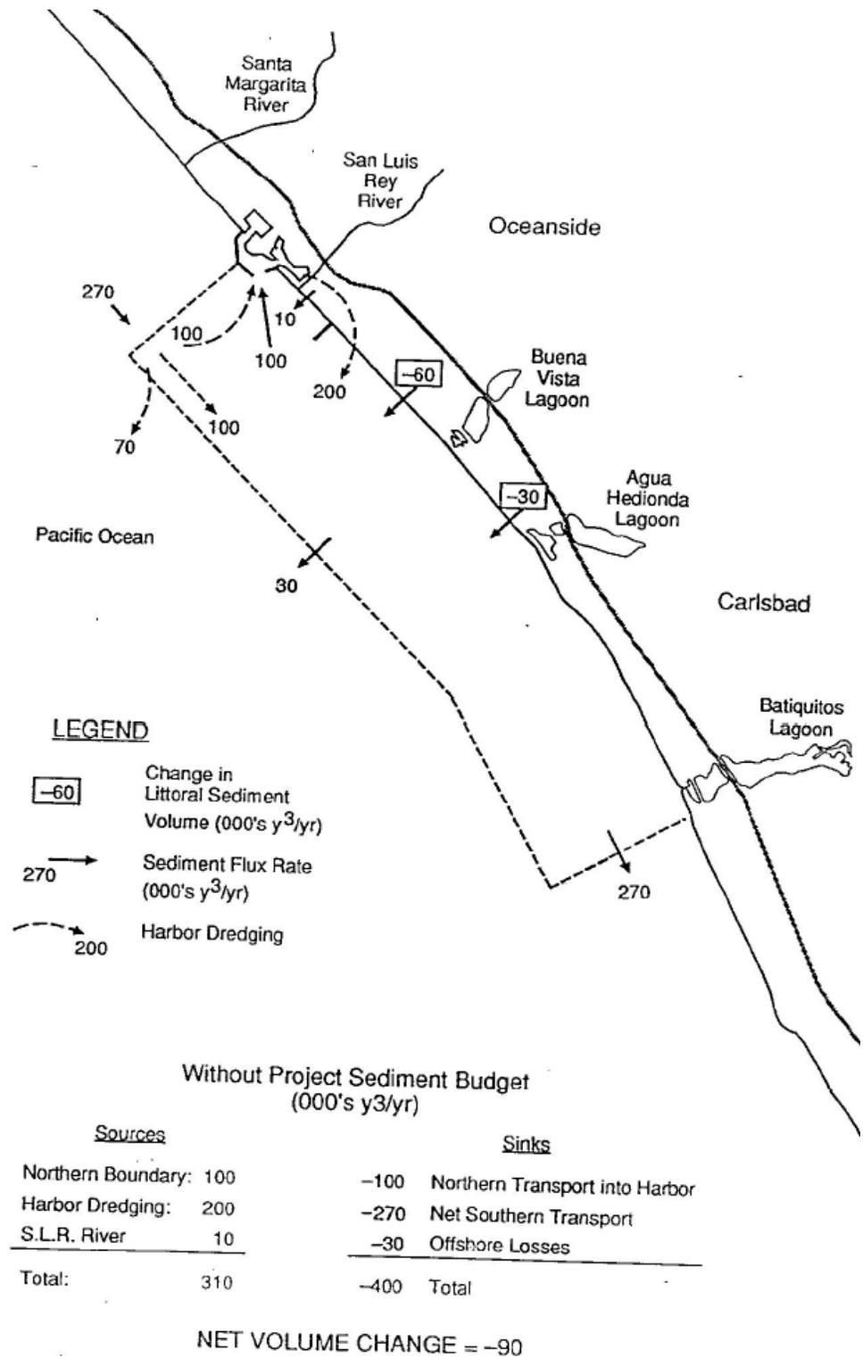
**Figure 2-5. Projected Sediment Budget for Oceanside (USACE, 1994)**
